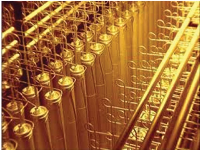
Gas centrifuges can be used to enrich uranium and are subject to nuclear nonproliferation (NP) controls.
